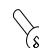
Bolt -4x12L, 2 EA :for Nozzle Holder -M4x12L, 2 EA :for Nozzle Holder, Gas Valve
